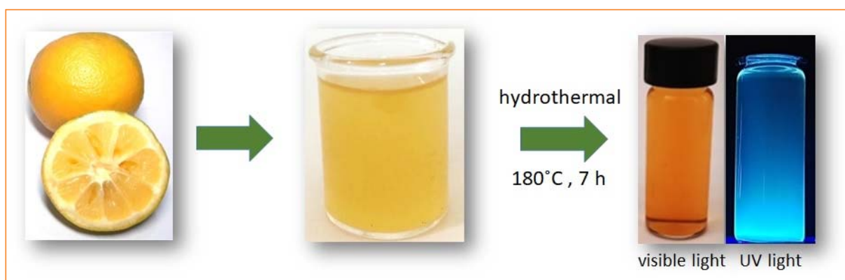
Figure 1: Schematic illustration of preparation of CDs from hydrothermal treatment of orange juice
