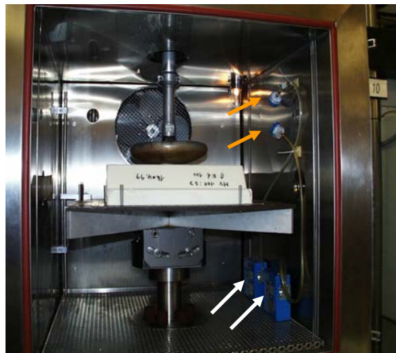
Figure 1: MDI-based polyurethane foam in the dynamic fatigue test chamber with air sampling pumps (white arrows) and sampling filters (orange arrows)
